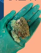
The metal whisks that were previously used in the studio to mix glazes caused scratches on the bottom of the glaze buckets. Switching to metal paddles led to the loosening of plastic from these scratches, contaminating the glaze with plastic particles.
